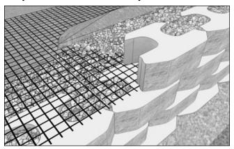
Place 3/4" to 1" clean aggregate (crushed rock) within the cores and a minimum of 12" behind the blocks. Place and compact backfill on the grid in lifts no greater than 8". When possible, it is recommended the backfill is deposited directly behind the wall and pushed to the end of the grid to ensure it remains taut and wrinkle-free.
