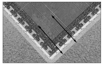
In the corner and on the next course of blocks, place a layer of grid perpendicular to the previous layer of grid. Repeat these steps for successive specified grid layers.
