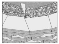
Slide the cap in place so that it is flush with the adjacent cap unit. Adhere caps with Super-Stik $^{\text{\tiny TM}}$ .
