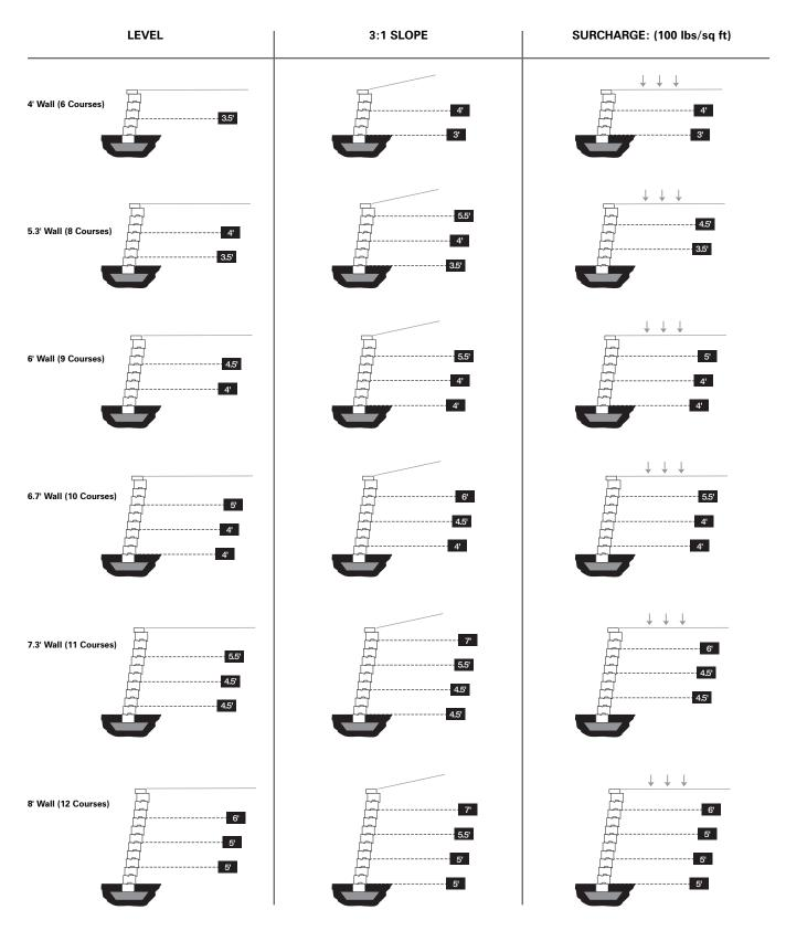
Friction angles (φ); (φ)=32 degrees for Silty Coarse Sand (SM). (φ)=28 degrees for Silty Sand/Sandy Silt (SM-ML). (φ)=24 degrees Clayey Silt/Silty Clay (ML-CL).
