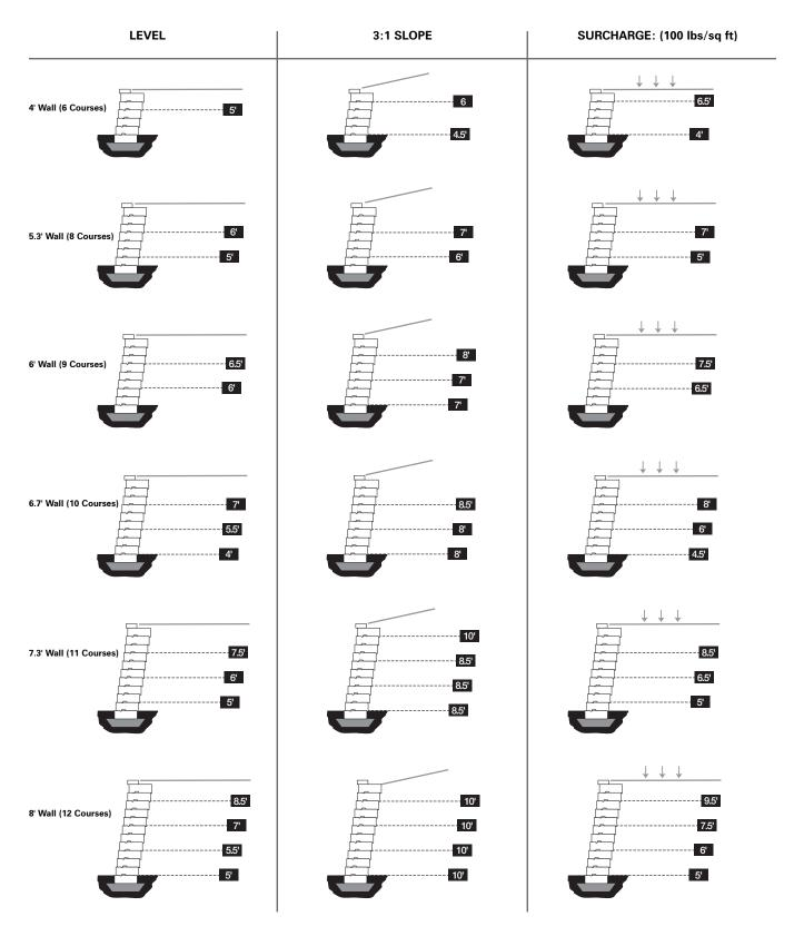
Friction angles (φ); (φ)=32 degrees for Silty Coarse Sand (SM). (φ)=28 degrees for Silty Sand/Sandy Silt (SM-ML). (φ)=24 degrees Clayey Silt/Silty Clay (ML-CL). Designs assume a 6" compacted angular aggregate base (road base) leveling pad and swale directly behind wall. Rockwood's design charts are for preliminary use only. A final site specific design should be evaluated and approved by a qualified professional engineer.
