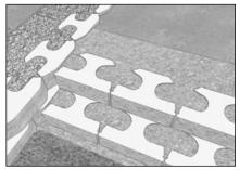
previous riser by 2". Fill the cores and backfill behind the wall with the base material to 95% Standard Proctor. Repeat this process for each successive riser. The side stair walls must be vertical with no setback.
