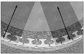
Place grid following the contour of the curve.
