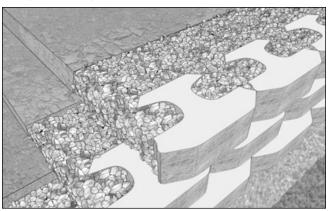
The area behind the wall on the grid layer needs to be level with the top of the block and to 95% of the Standard Proctor (ASTM D698).
