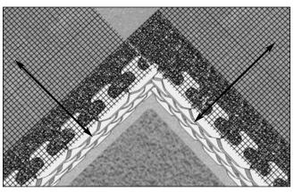
At the next designed grid layer, alternate the edge on which the grid is extended past the corner. Repeat these steps for successive specified grid layers.
