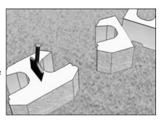
To create a Corner Block, make score lines on both splitting grooves and behind the head of the block. Split the block on both top and bottom sides, as shown. A hammer and chisel, or a
