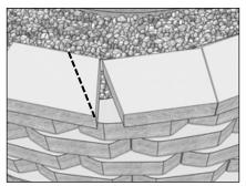
Using this measurement, cut the cap so that it is parallel with the adjacent cap unit.
