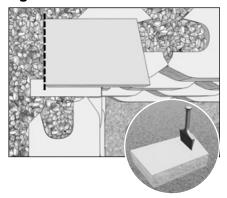
Cut the next Universal Cap to be flush with the corner cap. Adhere Universal Caps with Super-Stik™.
