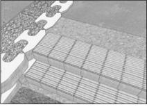
Proper compaction to 95% Standard Proctor is crucial in a stair step application. Each successive Step Tread should overlap the previous riser by 2" to 5". Repeat this process for each successive riser. The side stair walls must be vertical with no setback.
