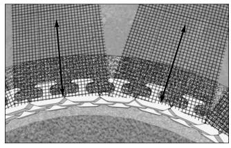
After the next course of block is placed, lay the grid to cover the area of unreinforced soil below. This will ensure 100% coverage. Repeat these steps for successive specified grid layers.
