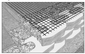
Place the grid as close to the face of the wall without exposing it after successive placement of blocks. Ensure the grid is placed with the strength direction perpendicular to the wall. Check grid manufacturer specifications for proper grid placement instructions.
