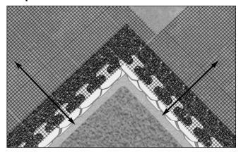
Extend the grid past one edge of the wall by a minimum of 2'. Along the other edge, place the grid to the corner.
