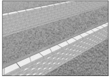
tiered walls independently, the walls must be set back a distance of at least twice the height of the lower walls. Whenever tiered walls are constructed, a qualified soils engineer should be consulted.
