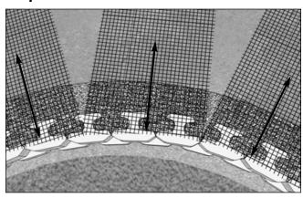
Making sure the strength direction of the grid is perpendicular to the wall face, align the cut grid sections so they follow the contour of the concave curve. Grid layers should not overlap. An engineer will specify the length of grid.
