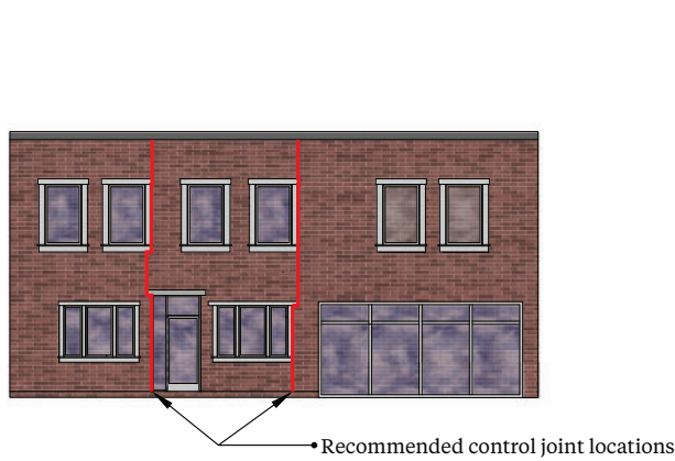
FIGURE 9—Example of Veneer Control Joint Placement
